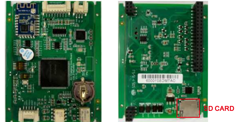
Micro SD slot of 7kW charger
